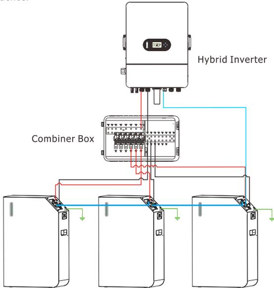
Figure 4-1 The parallel connection of three battery packs
