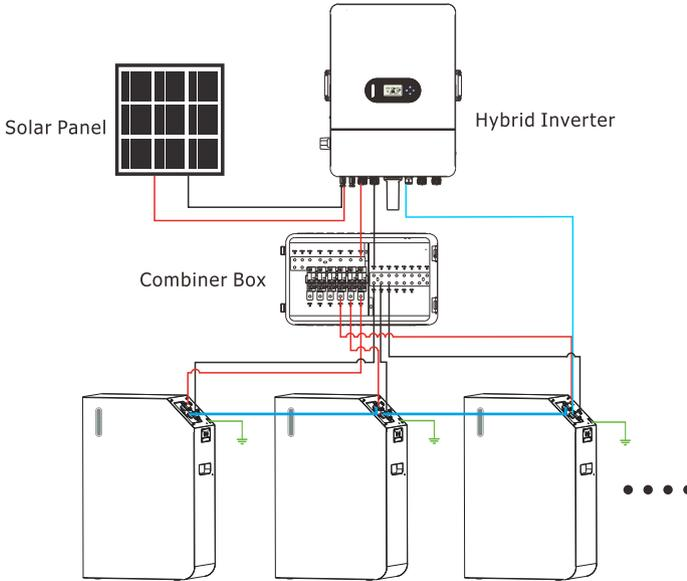
Figure 3-2 Multiple Battery Parallel System Connection Diagram
