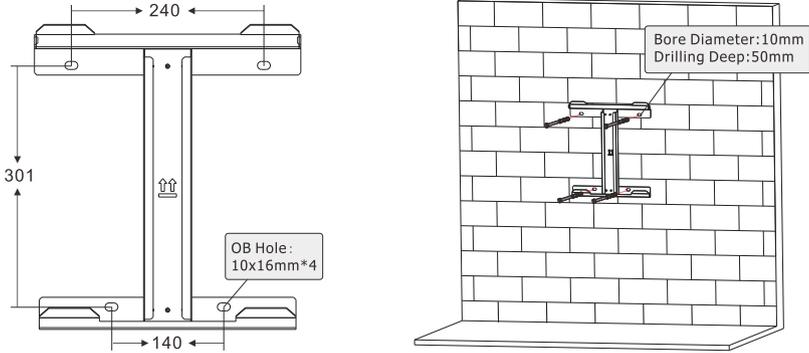
Step 2: Lift the machine onto the wall mounted components to secure it, Lock one M4\*12 screw on the left and right sides of the wall mount.
